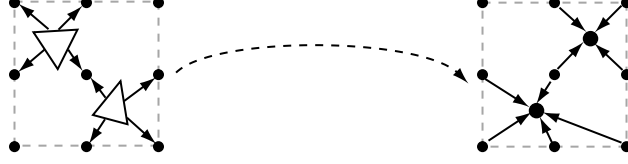
Figure 3-7: Schematic of the FFTSVD method for computing long-range interactions.
