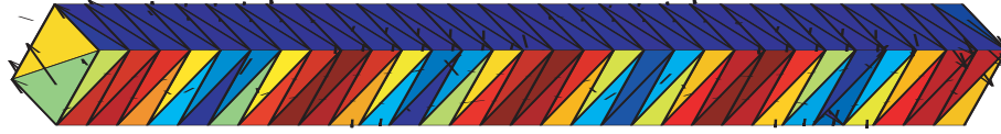
(s) Long thin wire. Over the frequency range, the wire has length .3\lambda to 3\lambda .
