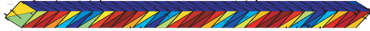
(a) Long thin wire: Over the frequency range, the wire has length .3\lambda to 3\lambda .
