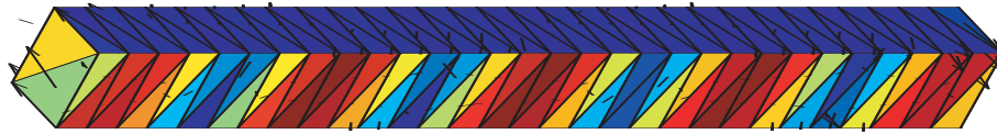
(a) Long thin wire. Over the frequency range, the wire has length .3\lambda to 3\lambda .
