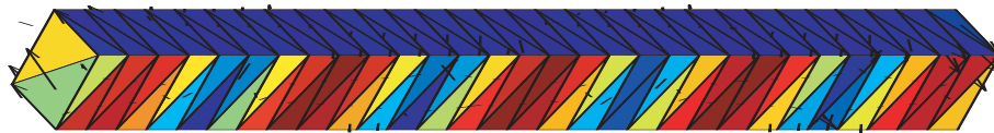
(g) Long thin wire. Over the frequency range, the wire has length .3\lambda to 3\lambda .
